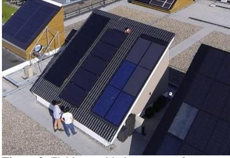
**Figure 2:** Field test with three types of uncovered PVT systems on the dummy roof in the middle
