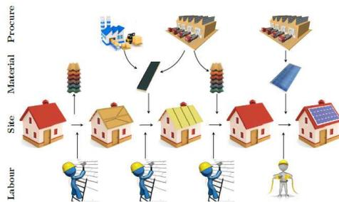
**Figure 1** Schematic representation of the traditional roof renovation process involving PV, consisting of the steps roof tile removal, insulation installation, roof tile installation and PV installation.
