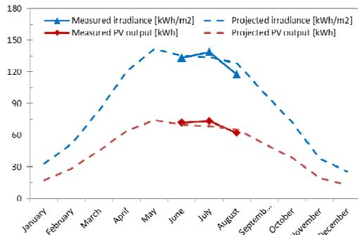
**Figure 8** Projected versus measured irradiance [kWh/m<sup>2</sup>] and energy output [kWh] for the prototype insulation integrated PV element equipped with micro-inverters.
