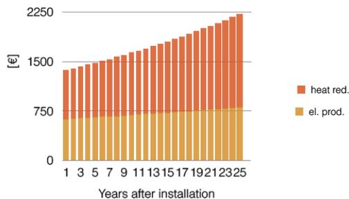
**Figure 6** Annual cost savings in euro for a typical Dutch house built before 1974, after renovation of the roof with roof insulation integrated PV. The cost savings are split up in insulation related heating savings and PV-related electricity savings.
