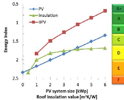
**Figure 4** Effect on the Energy Index (left y-axis) and Energy Label (right y-axis) of a typical Dutch terraced house built before 1974. Shown is the effect of the application of a PV system (blue line), the insulation of the roof (green line), and the combined Insulation Integrated PV on the roof (IIPV – red line).
