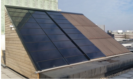
Fig. 2. The modules on the left hand side operate under MPP and were connected to micro inverters and power meter ('AC test') while the central and right hand modules were connected to an IV tracer ('DC test').
