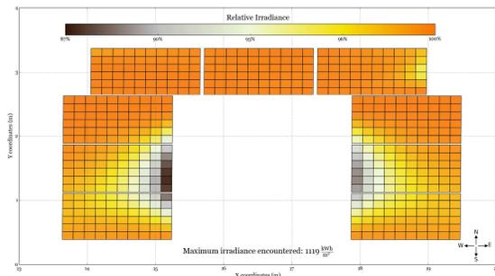
Figure 6: Annual irradiance reduction due to shading for the modelled roof
