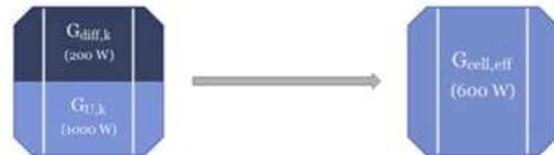
Figure 4: Principle of deriving the effective cell irradiance from its shaded and unshaded fractions. In this example,  $\sigma_P = 50\%$ . Modified from previous similar work (Sinapis, et al., in press; Tzikas, 2015)
