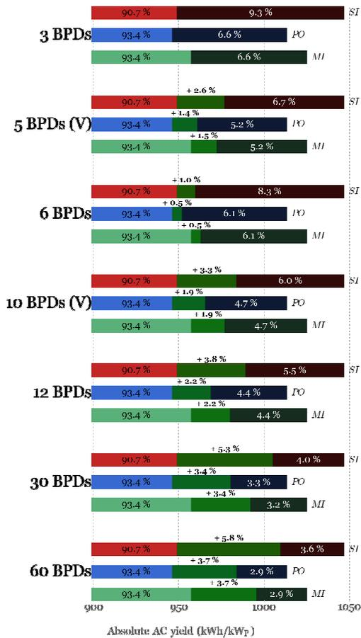
Figure 9: TMY AC yield results for SI(+), PO and MI systems. Shading index values and potential benefits when increasing the amount of BPDs per module in a stepwise fashion from 3 to 60 are illustrated
