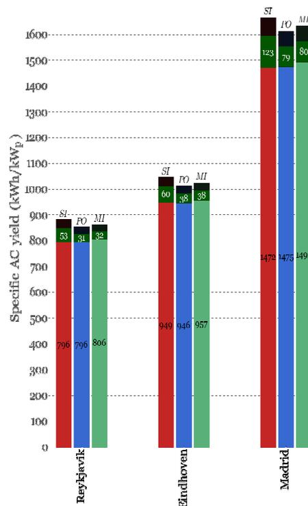
Figure 10: Specific AC yield results for SI(+), PO and MI systems placed in Reykjavik, Eindhoven and Madrid. The red, blue and light-green bars and the corresponding black text indicate the 3-BPD reference specific AC yield in kWh/kW<sub>p</sub>. The dark green bars and the corresponding white text indicate the potential benefits in kWh/kW<sub>p</sub> if 60 BPDs per module are used instead of three
