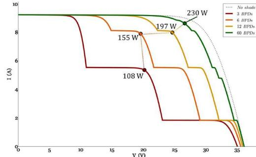
Figure 8: IV responses of example module under partial shading as in Figure 7. The cases of 3, 6, 12 and 60 per-module BPDs are shown. All increases lead to increases in extractable power, as can be seen from the highlighted MPP-values. The grey dashed line represents the IV curve in unshaded conditions. Total irradiance: 1000 W/m<sup>2</sup>; diffuse irradiance: 200 W/m<sup>2</sup>; T<sub>mod</sub>: 40 °C
