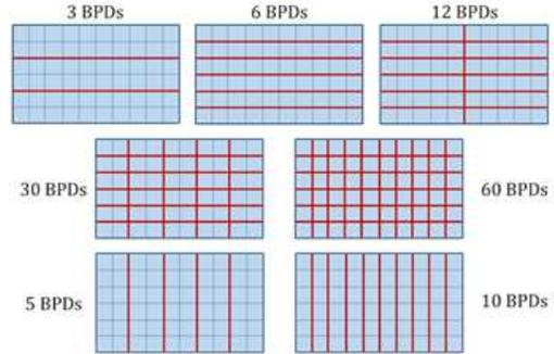
Figure 3: Substring granularities or variation of per-module BPDs investigated in this research. The 3, 6, 12 and 30 BPD cases are referred to as horizontally aligned substrings; the 5 and 10 BPD cases as vertically aligned substrings. Bypass diodes per cell are assumed in the 60 BPD case
