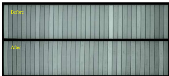
Figure 8: EL image of the CIGS_A module before the shading stress was applied (top image) and after the shading stress was applied (bottom image).
