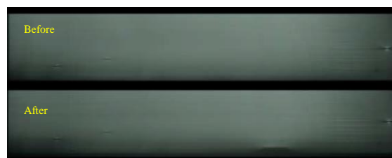
Figure 14: EL image of the masked side of the CIGS_G module before and after the shading stress respectively
