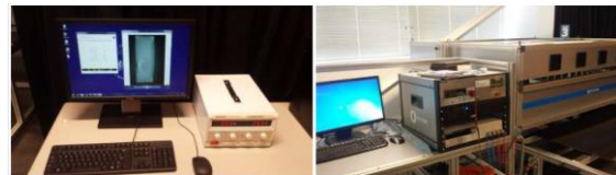
Figure 2: Electro-luminescence equipment, I-V tracer and solar simulator used for the experiments
