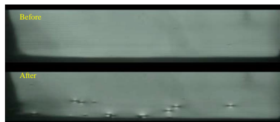
Figure 10: EL image of the masked side of the CIGS_C module before and after the shading stress respectively
