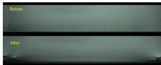
Figure 13: EL image of the masked side of the CIGS_F module before and after the shading stress respectively
