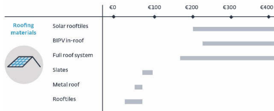
Figure 6: Cost of BIPV roof tiling compared to other roofing materials used in conventional pitched roof.
